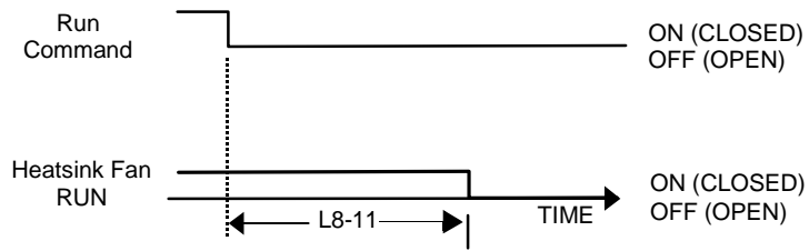
Fig. 84 Heatsink Cooling Fan Operation Timing Diagram
